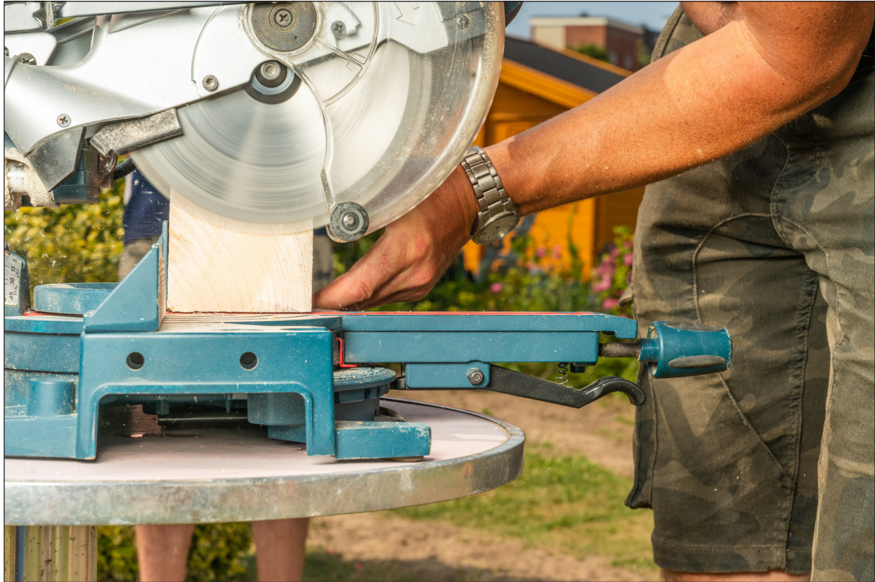
Figure 1. A carpenter saws a wooden beam without protective equipment. In a performance test, use of personal protective equipment is likely a gating item. The candidate would fail immediately, notwithstanding any carpentry skills he may possess.
